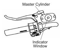
4. If the fluid level is low add DOT 4 brake fluid only. Do not overfill.
